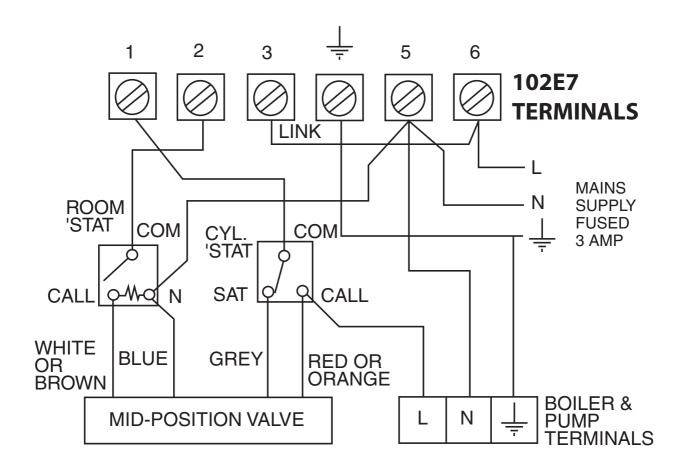
The above control system is available as the Danfoss Randall 102E7 HEATSHARE pack, which also includes the RMT room thermostat, AT cylinder thermostat, HS3 mid-position valve and a WB12 wiring box.
