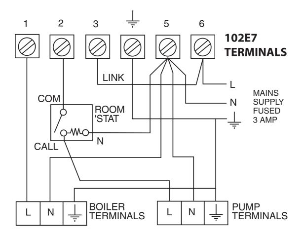
Typical domestic gas or oil-fired central heating system with gravity hot water and pumped heating. (If a room thermostat is not used, wire pump live directly to terminal 2 of the 102E7).
